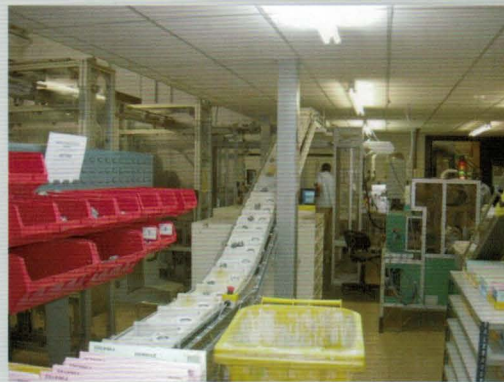
Friction Chain Decline up to 25°
